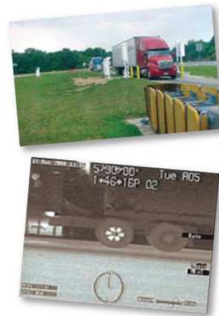
Top, each vehicle is scanned as it passes through ISSES scanners and data is passed to a computer located in the scale house. Bottom, an example of the Infrared Image that is displayed on a video terminal located in the weigh station.
