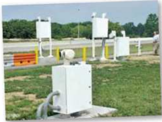
The Infrared camera passes the Infrared and color image to a video terminal located in the weigh station.
